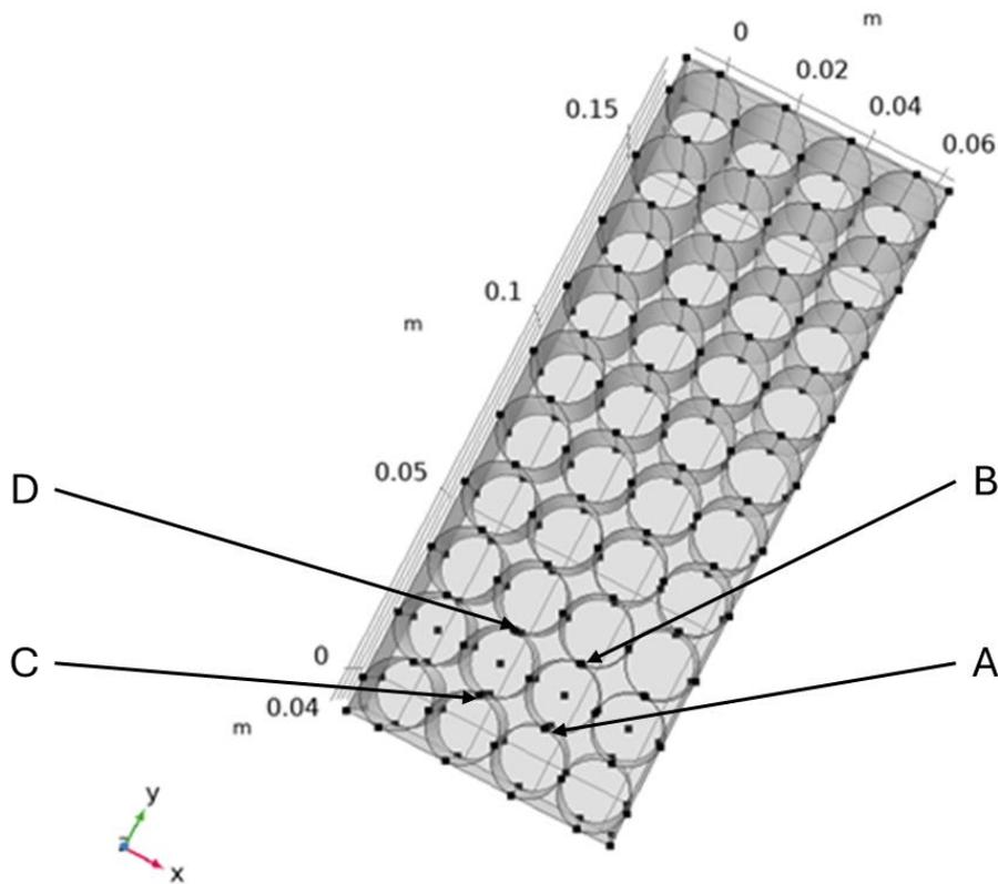
Figure 6. Temperature measuring points in the module.
