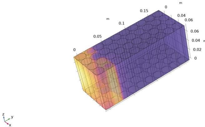
Figure 8. Temperature distribution in the battery cells where one cell ejected out of the battery module (Replaced with an air pocket.) after 480 seconds.
