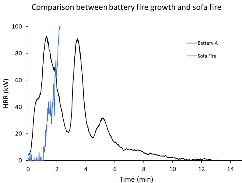
Figure 11. Comparison of experimental HRR from test on Battery A vs Sofa Fire
