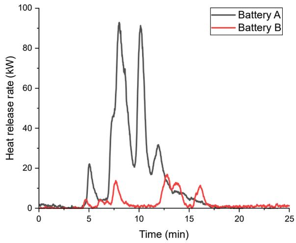
Figure 4. HRR curves from test 5 (battery A) and test 8 (battery B).
