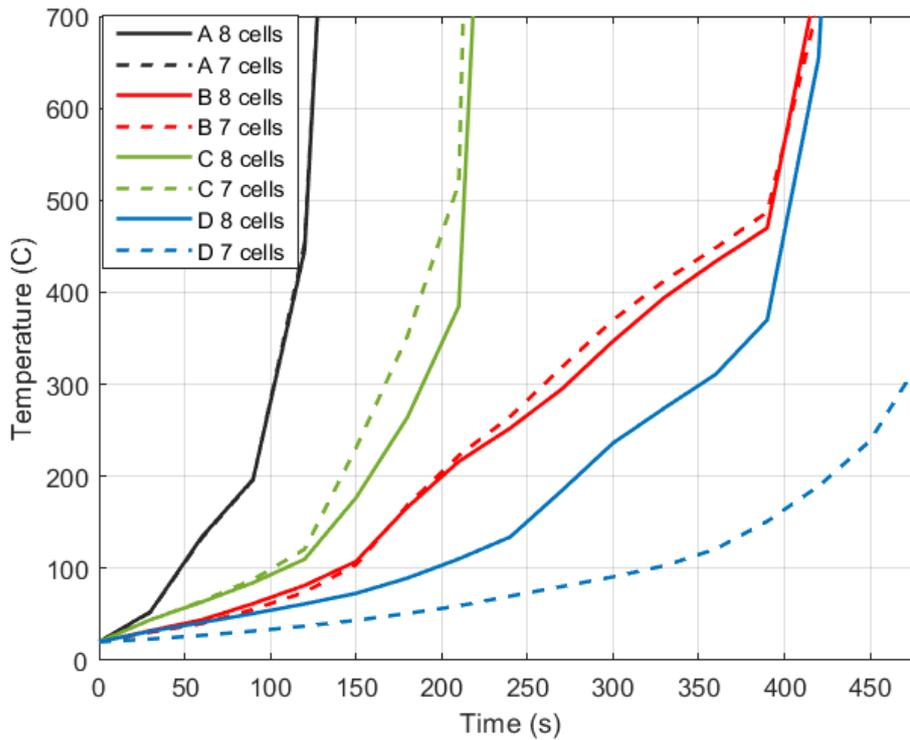
Figure 9. A comparison of the temperature history of the cases with 7 (dashed lines) and 8 (solid lines) cells in locations A, B, C and D according to Fig. 6. The difference in temperature rise is significant in the case where the blue dashed line (7 cells) lags behind the solid line (8 cells).
