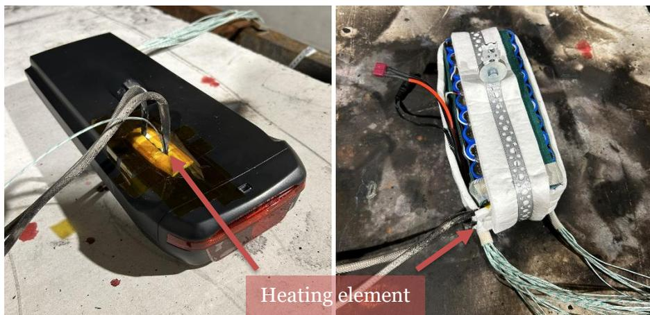
Figure 2. Battery A (left) and B (right) prepared for testing with installed heating element as well as temperature and voltage measurements.
