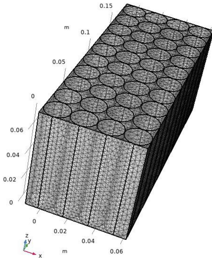
Figure 5. A typical coarse mesh for the module with air.
