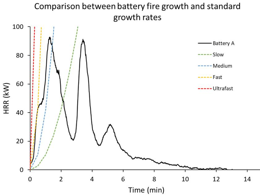
Figure 10. Comparison of experimental HRR from test on Battery A vs standard growth rates
