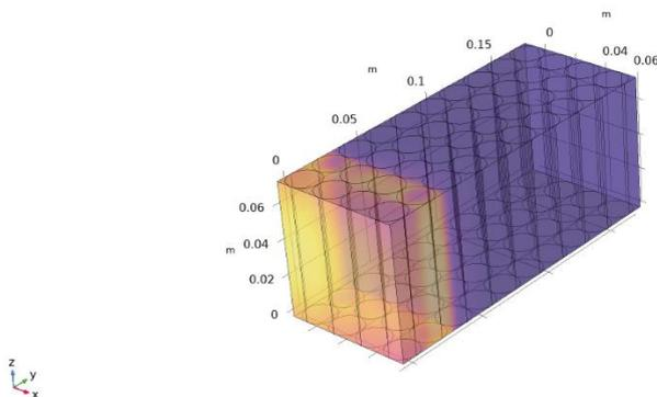
Figure 7. Temperature distribution in the battery cells after 480 seconds where 8 cells are assumed to go to thermal runaway.
