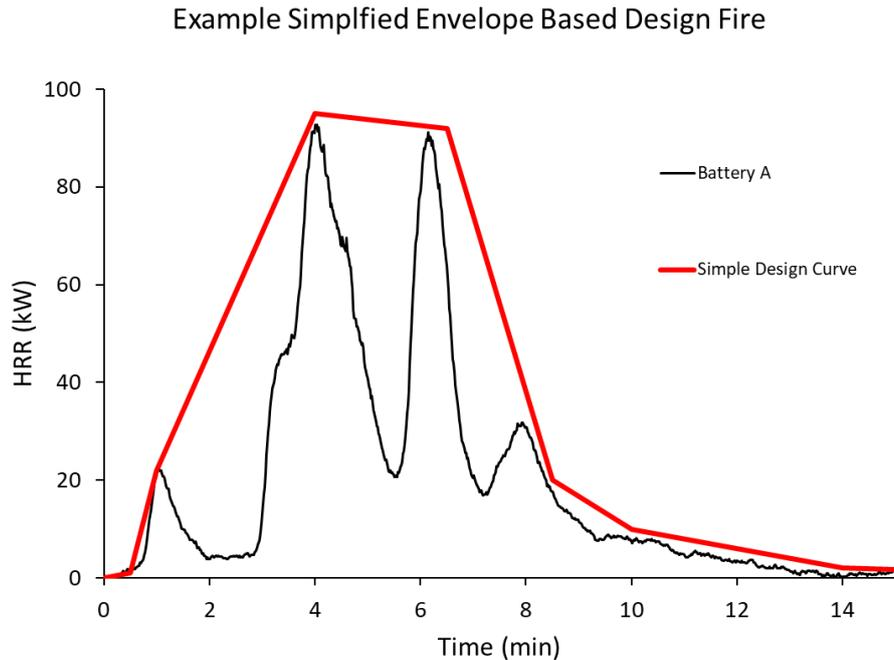
Figure 12. Example of a simplified design curve based on an envelope over the Battery A test results.
