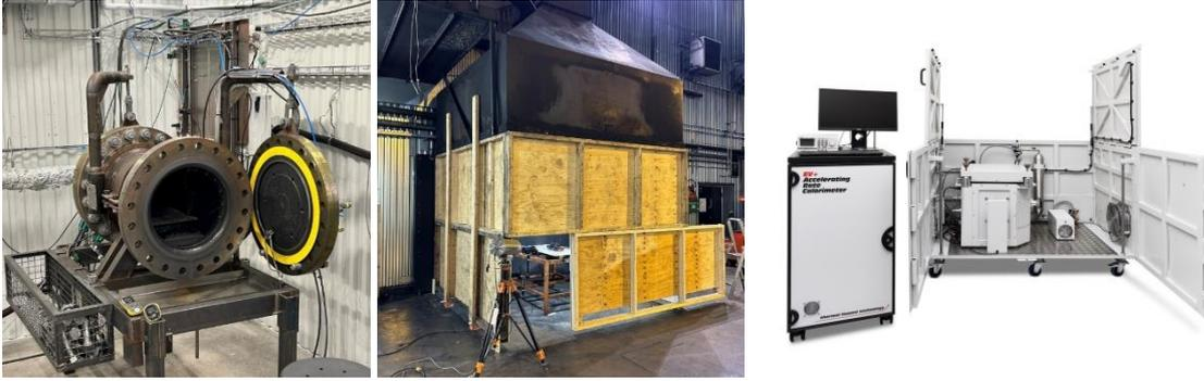
Figure 3. Closed pressure vessel setup with inert atmosphere (left), open setup below an exhaust collector hood (middle), and standard ARC setup (right).
