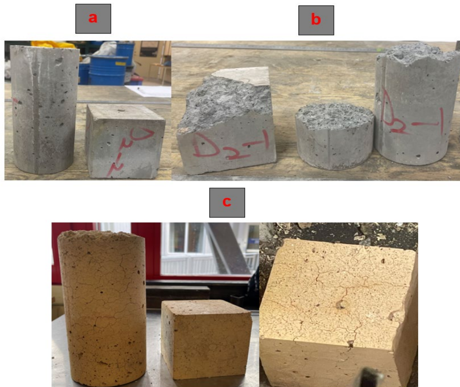
Figure 6: Concrete samples exposed to a) 200 °C b) 600 °C c) 1000 °C
