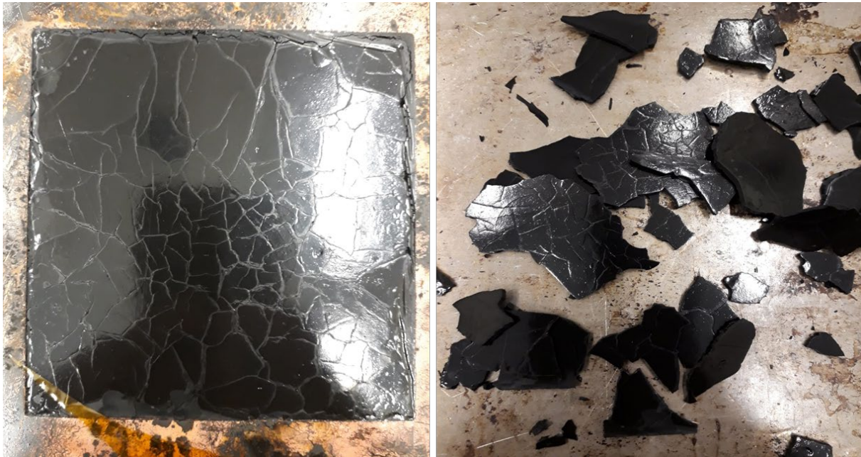
Fig. 4. The BC_APP_PA 11_COMP sample right after compression moulding. The sample inherently did not fuse and when it was taken out of the mould, the plate shattered. Several attempts gave the same result.
