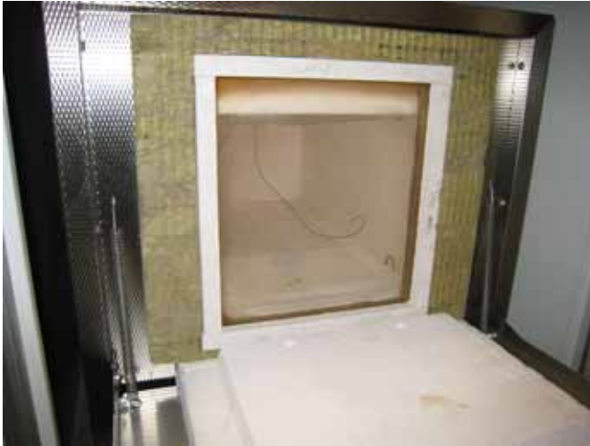
Figure 1. Furnace and the pane of fireproof glass
