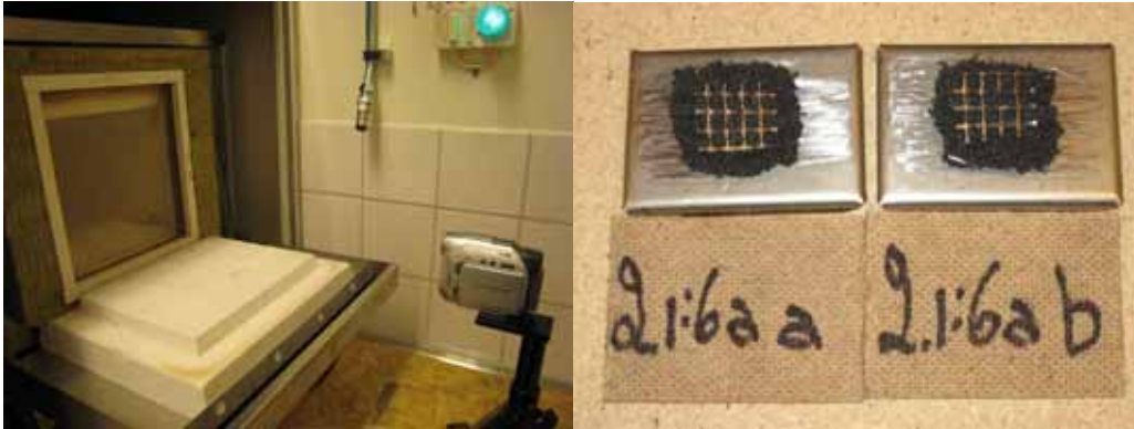
Figure 5. Video recording and photographing of samples after heating
