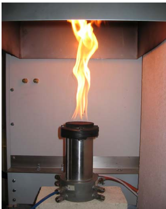
Figure 8. The McKenna burner with propane flame under the hood of the cone calorimeter.
