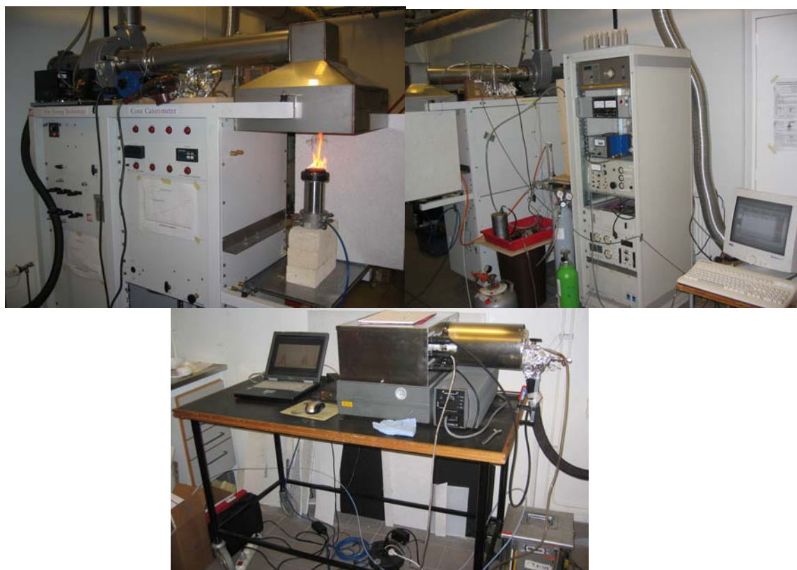
Figure 9. The experimental set-up used when measuring thermal breakdown of extinguishing agents.
