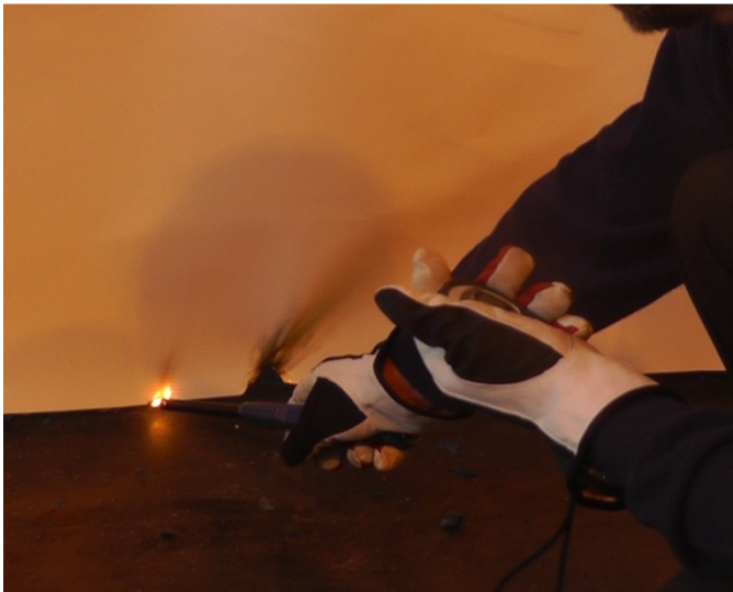
Figure 67 Ignitability tests with edge exposure.
