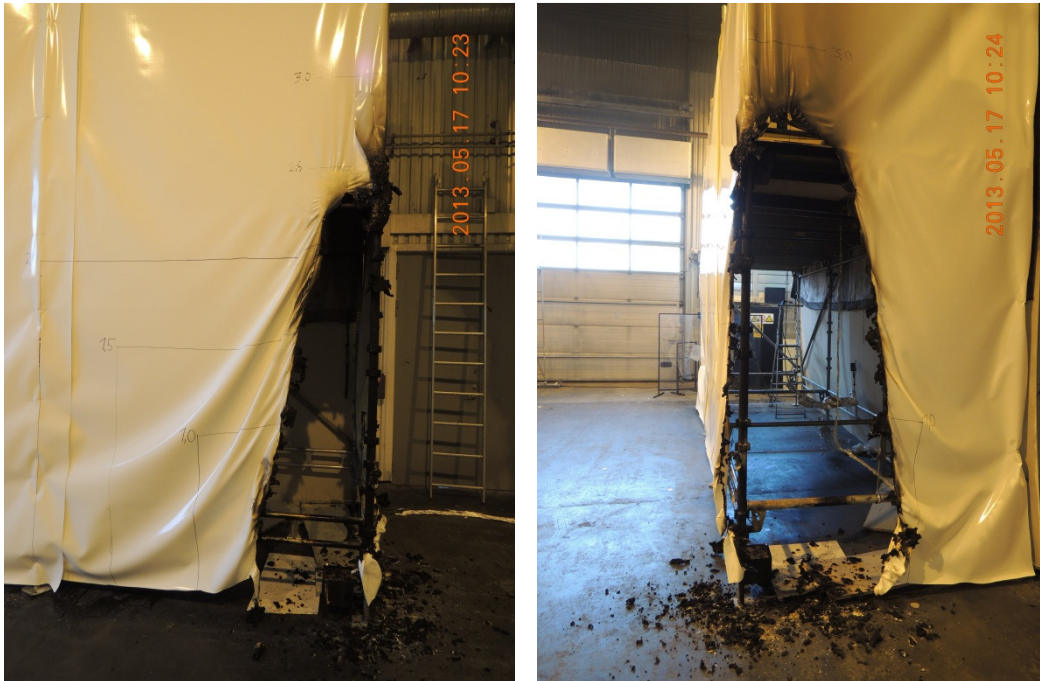
Figure 61 Fire damage of the material after the burner was turned off (left: front side | right: short side).
