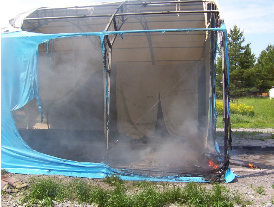
Figure 12 Damages to the test building as documented after the test.
