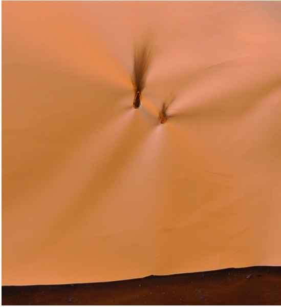
Figure 71 Fire damage after surface exposure at the outside (right: 15 s flame exposure; left: 30 s flame exposure).
