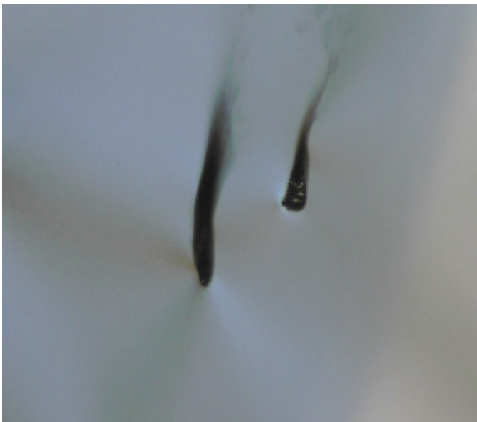
Figure 76 Fire damage after surface exposure at the inside (right: 30 s flame exposure; left: 15 s flame exposure).
