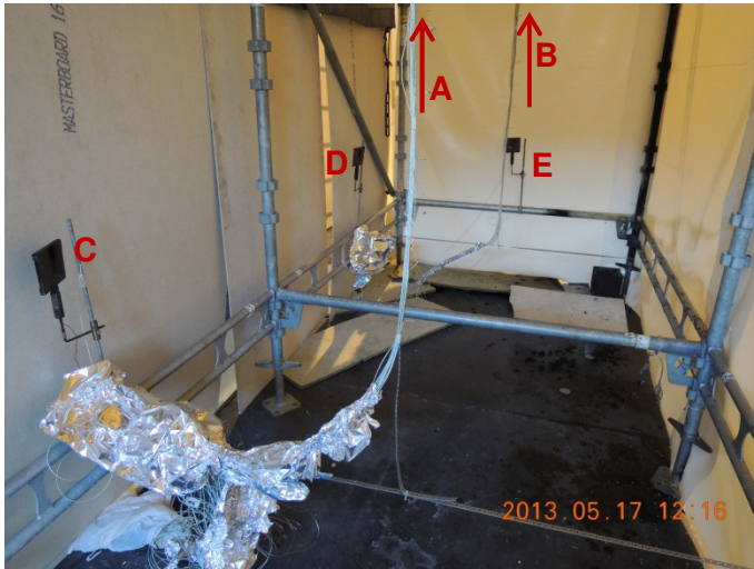
Figure 27 Thermocouple trees (position A and B) and plate thermometers (position C, D and E).
