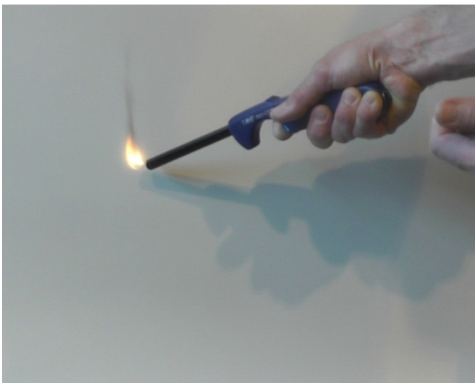
Figure 68 Ignitability tests with surface exposure.
