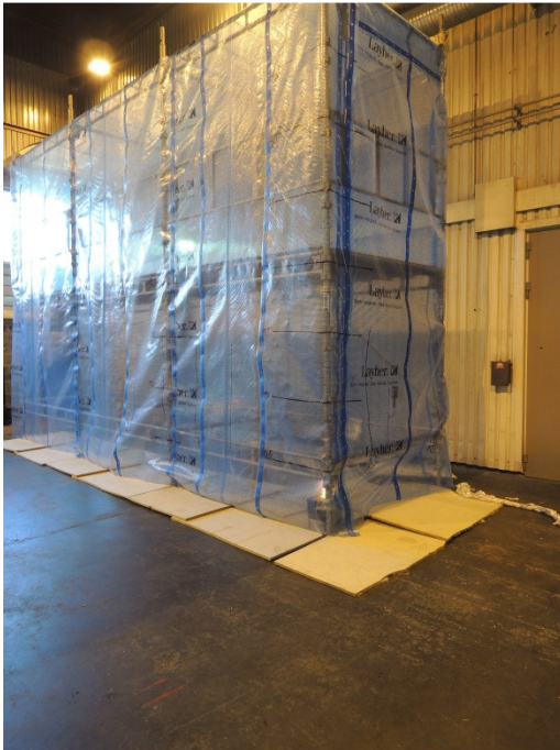
Figure 16 Front side and the short side exposed to the ignition source.
