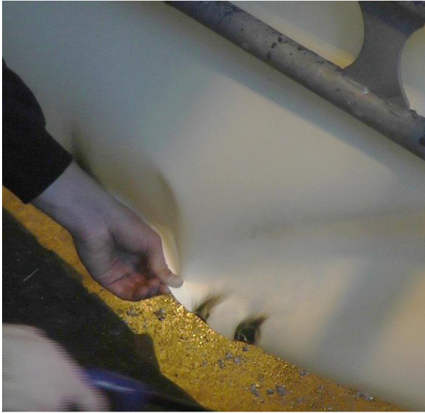
Figure 74 Fire damage after edge exposure from the inside (right: 30 s flame exposure; left: 15 s flame exposure).
