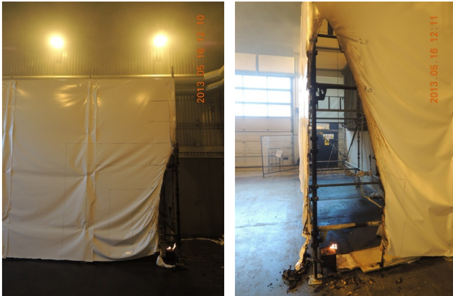
Figure 43 Fire damage of the material after the burner was turned off (left: front side | right: short side).
