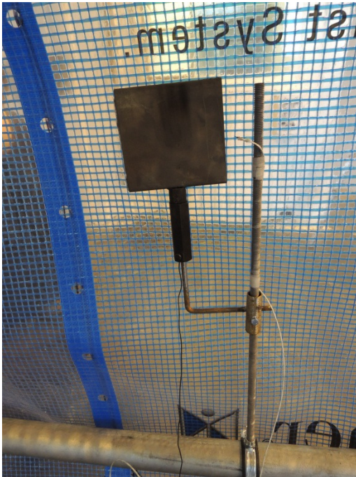
Figure 26 One of the plate thermometers and the reference thermocouple (white wire).
