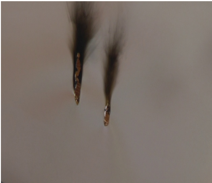
Figure 72 Fire damage after surface exposure at the inside (right: 15 s flame exposure; left: 30 s flame exposure).
