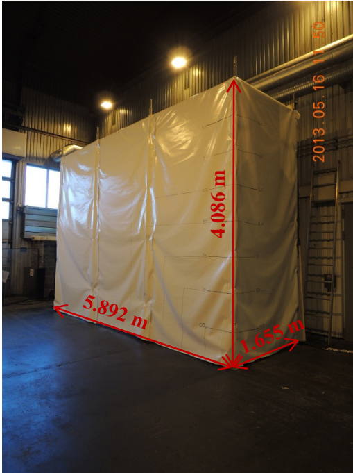
Figure 19 Front-side and the short side exposed to the ignition source.
