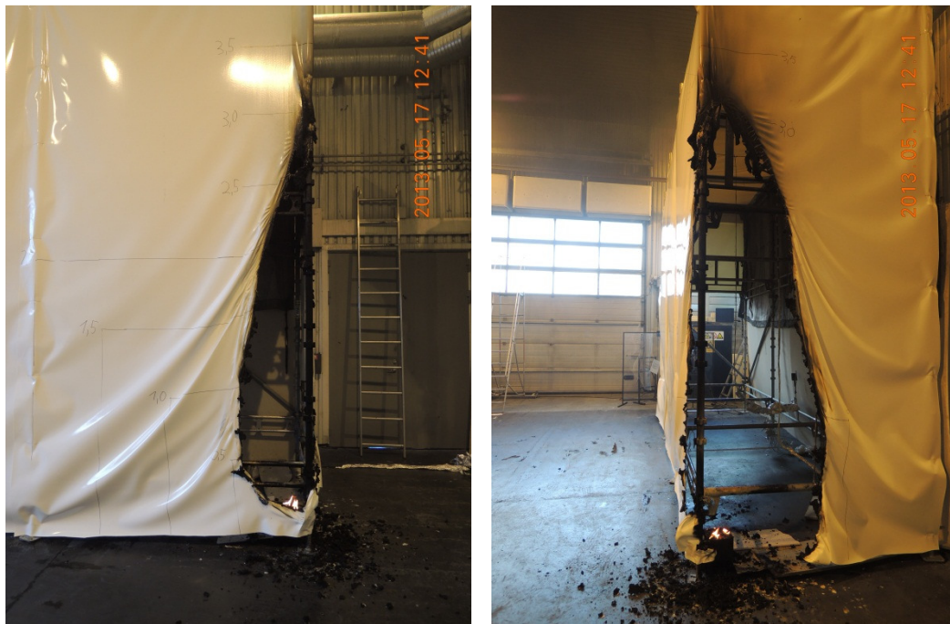
Figure 49 Fire damage of the material after the burner was turned off (left: front side | right: short side)
