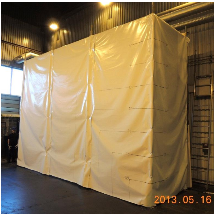
Figure 28 Markings for flame spread observations.
