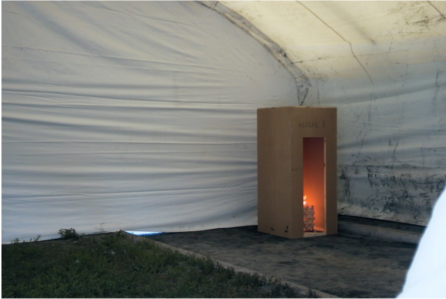
Figure 10 The fire source placed in a corner of the tent building (just ignited).
