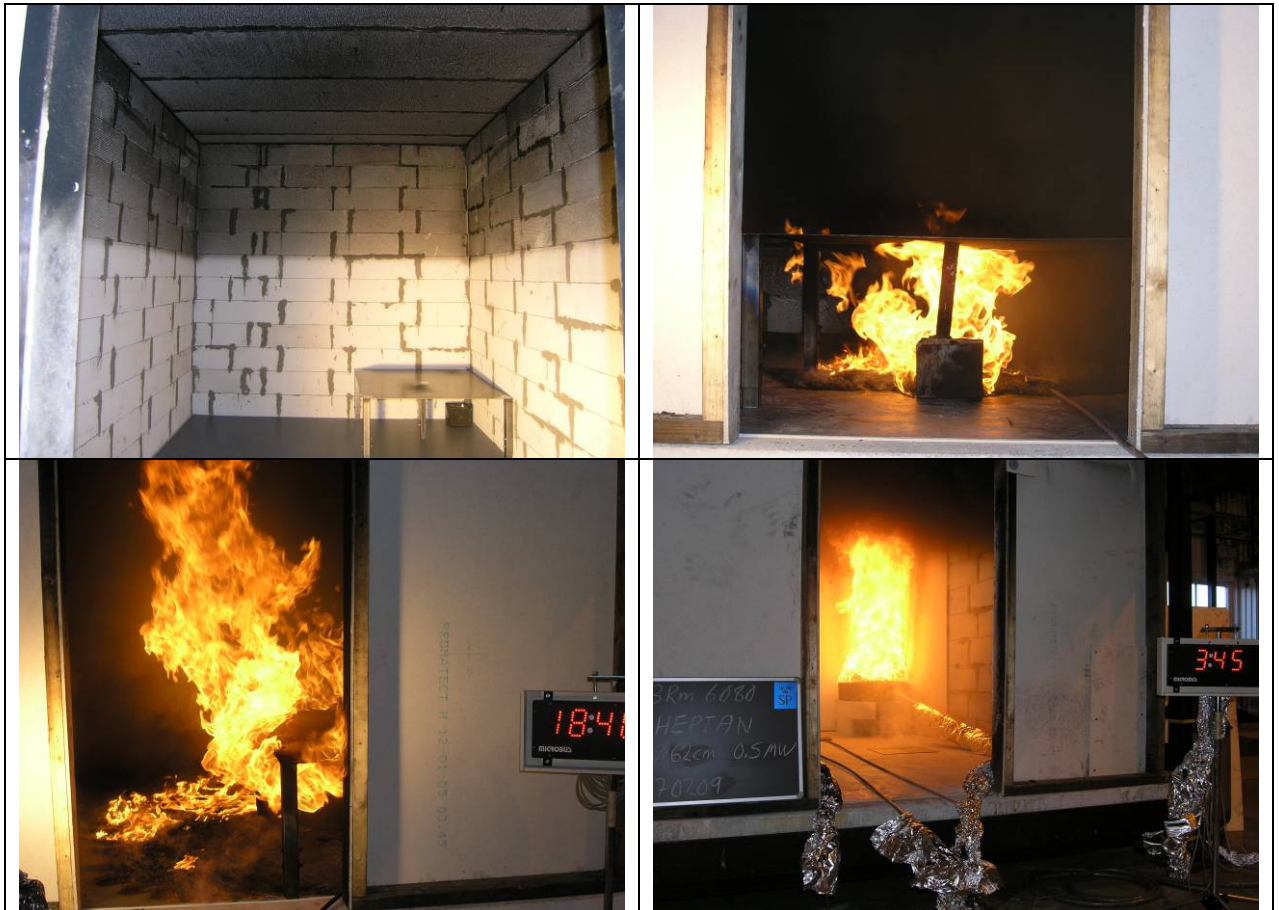
Figure 6 Room/Corner test set-up/experiment in the 4 different project scenarios. Top row: scenario 1 and 2. Bottom row scenario 3 and 4.
