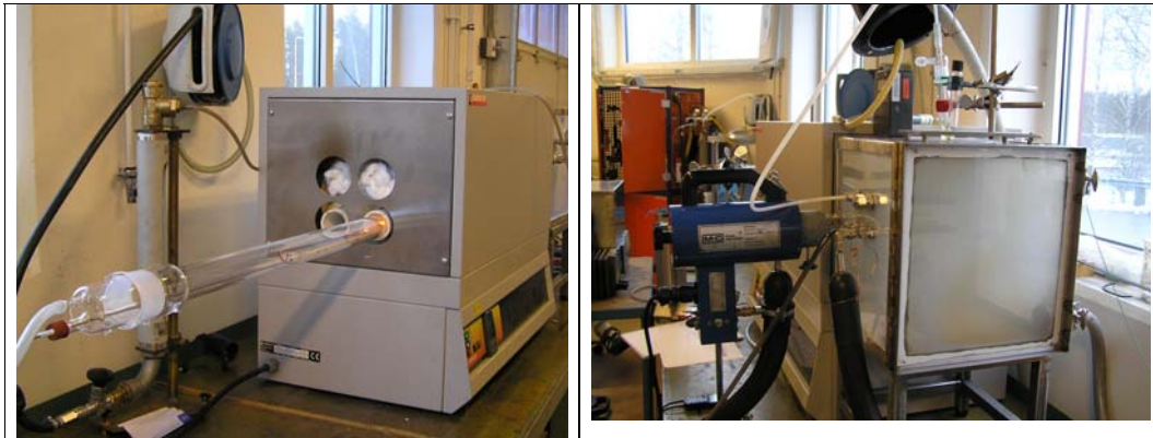
Figure 2 The Purser furnace from the front end (left photo), showing the quartz tube and primary air intake (plastic tube) and the back side with the mixing chamber (right photo)
