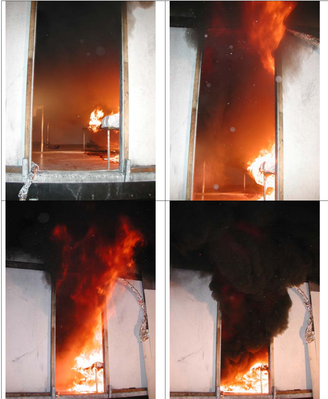
Figure 21 Sequence of photos showing how the mattress and the PVC floor-carpet together provokes a “local” flashover that makes the fire spread over the entire floor, inducing at the same time a full flash-over situation with heavy smoke.
