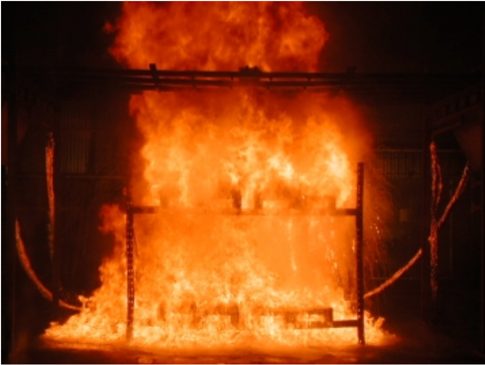
Figure D-11 The meltdown of the plastic (HDPE) containers during a test.
