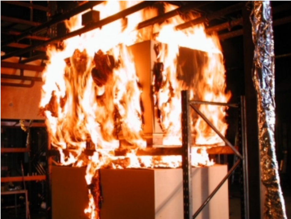
Figure D-10 The triple, bi-wall corrugated cardboard cartons (EUR standard class II commodity) during a test.
