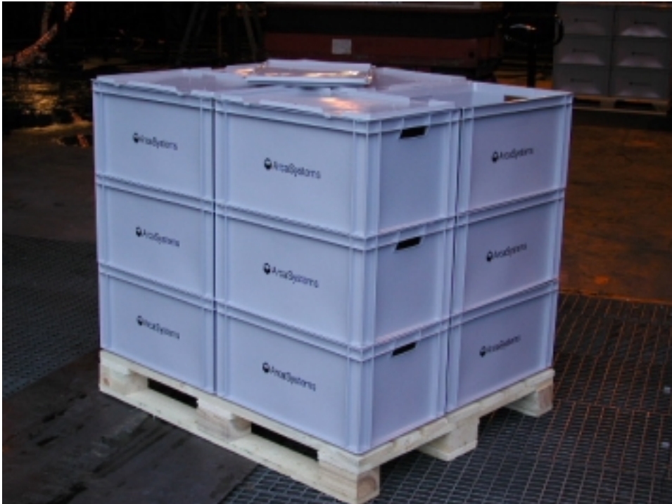
Figure D-3 Plastic (HDPE) containers. Each pallet load contained 15 pcs of containers. The top layer had a lid.
