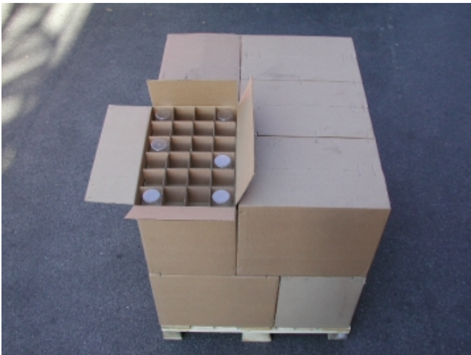
Figure D-2 The corrugated cartons with 15% (by weight) unexpanded plastic. Each pallet contained 300 pcs of polystyrene plastic cups. Note: The EUR standard plastic commodity is identical, except that plastic cups are placed in every compartment, i.e. 1200 cups per pallet load.
