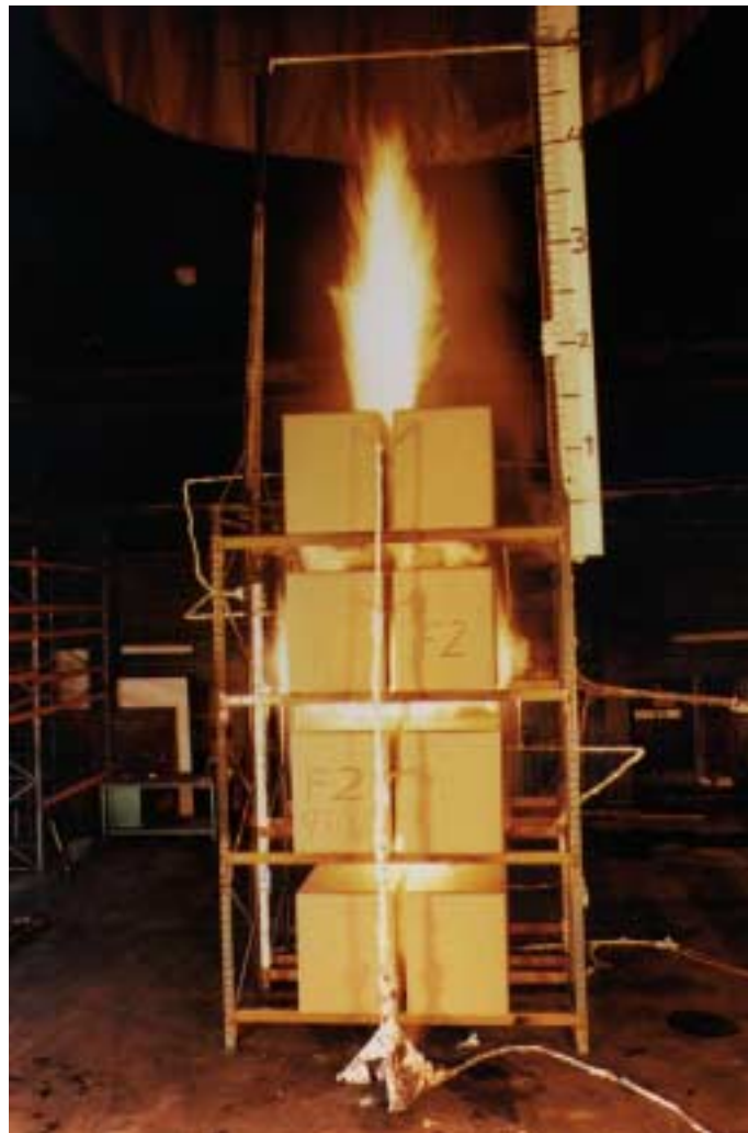
Figure 3 A large-scale experiment with Standard Class II material under the Industry Calorimeter at SP.
