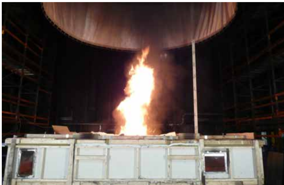
Figure 3.5 Photo with the scale model, flames from the ceiling opening, the height ruler, and the hood collecting the exhaust gases.
