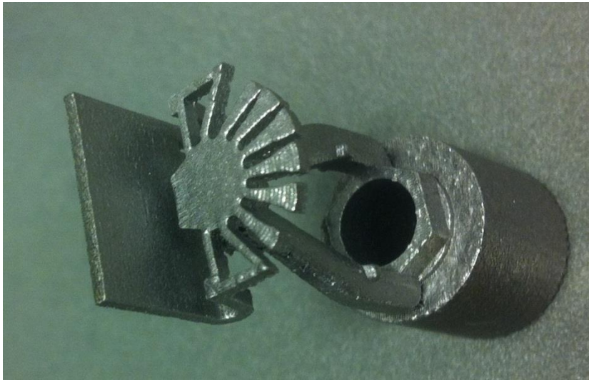
Figure 4 A photo of a 1:4 T-Rex nozzle that is made of steel.
