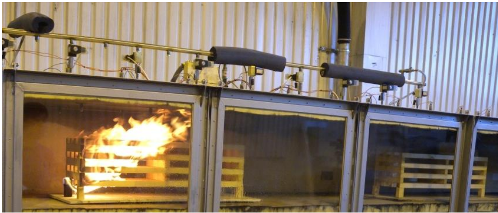
Figure 9 A photo showing a growing fire. The ignition source consisted of a fibreboard cube placed at the same level as the bottom of the wood crib and at the upstream edge of the wood crib. Another wood crib was placed downstream in order to investigate the risk for fire spread.
