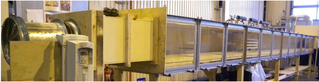
Figure 1 A photo of the 1:15 model scale tunnel using automatic sprinkler system. A fan was attached to the tunnel entrance and windows were placed along one side in order to observe the smoke flow and the flame volume.
