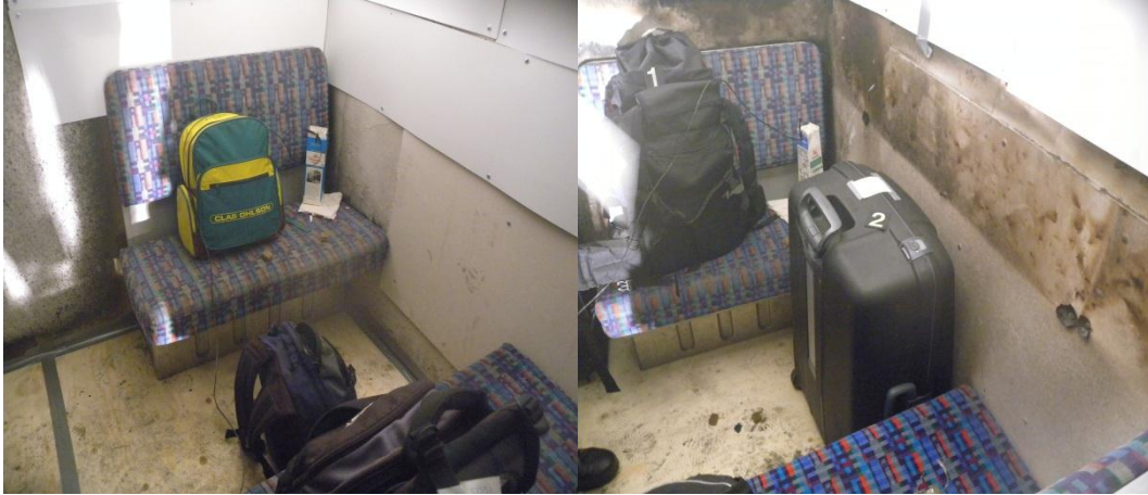
Figure 20 Disposition of bags in the vicinity to the ignition source in test 5 (left) and test 6 (right).
