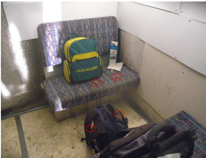
Figure 3 Picture from test 5 showing the experimental set-up with milk container filled with petrol. Positions of flames are marked with a red circle, the lower two were placed on the floor in front of the backpack.
