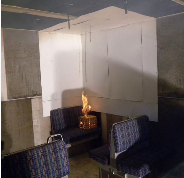
Figure 7 A photo of the HPL boards on the wall and ceiling above the ignition source.
