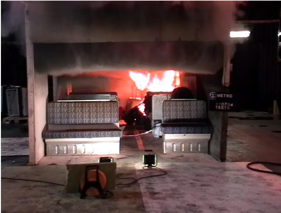
Figure 22 Test 6 shortly before a big piece of the burning HPL boards fell (time 1:21)
