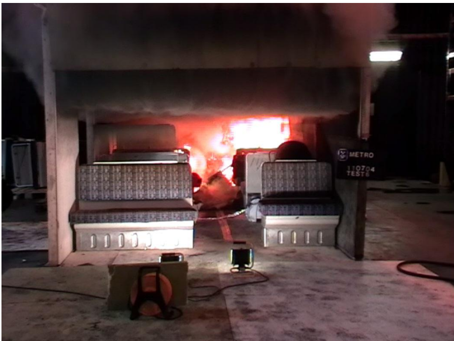
Figure 23 Test 6 shortly after a big part of the burning HPL boards fell (time 1:25). The HPL board fell at 1:23. The fallen HPL board can be seen in the middle of the carriage between seat S3 and S4.
