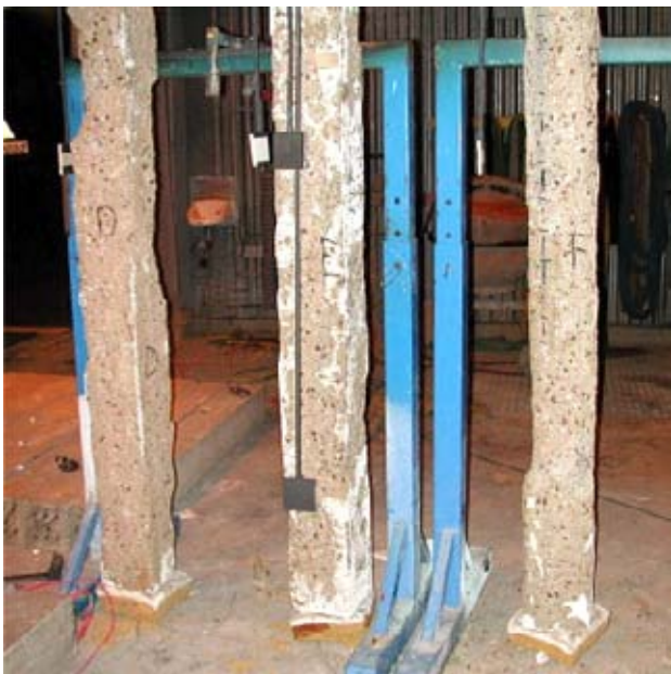
Figure B.4 Test specimens 40AG0-1, 40AR0-1 and 40AK0-2 from left to right.
