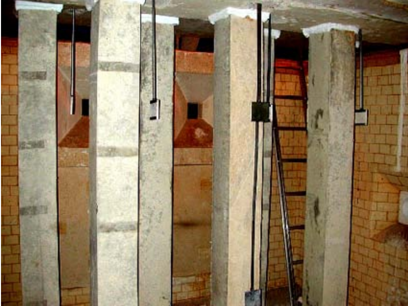
Figure B.1 Test specimens in the furnace before test.
