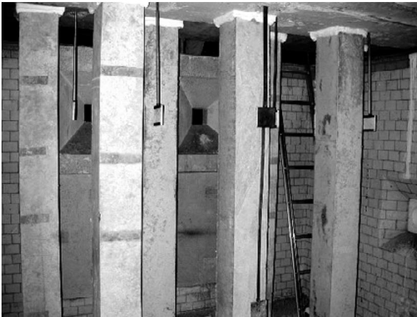
Figure 3.3 Test specimens in the furnace before test.
