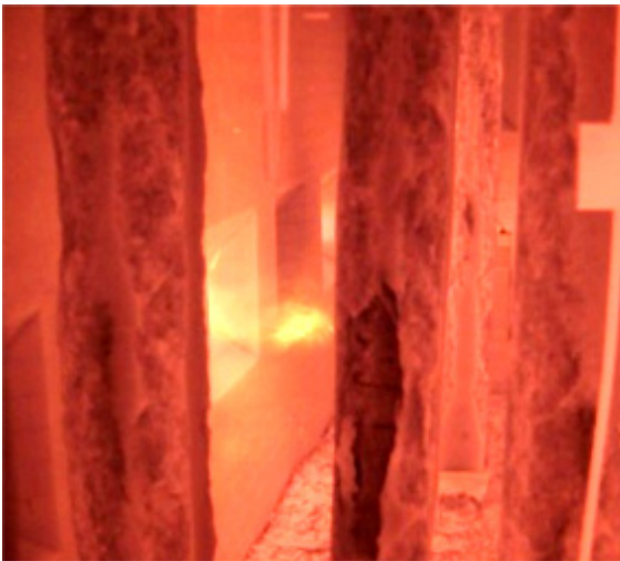
Figure B.2 Test specimens in furnace during test.
