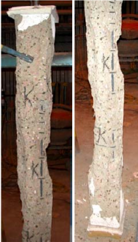
Figure B.9 Test specimen 40AK0-3.
