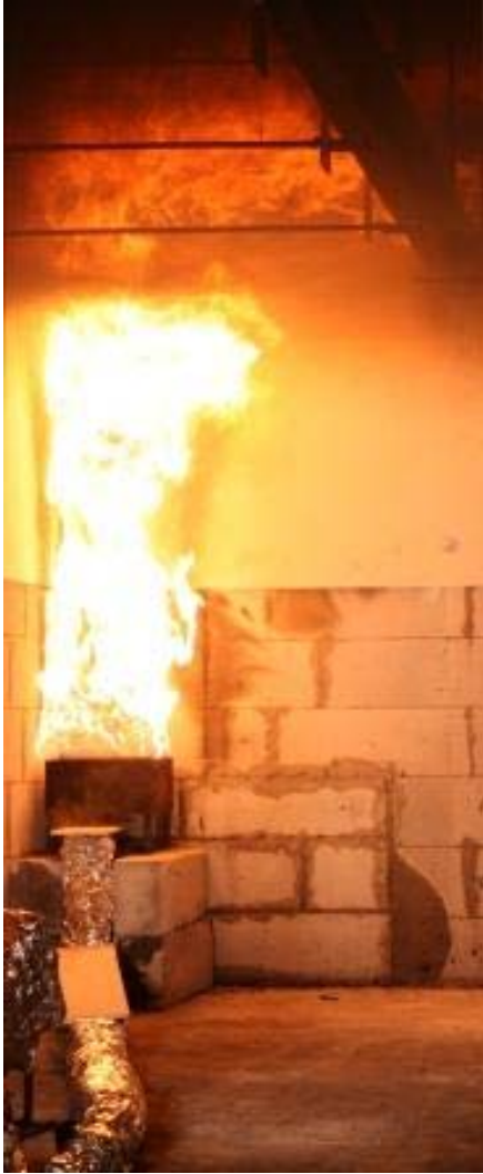
Figure 7 Elevated gas burner placed in a corner of the ISO 9705 Room/Corner test room.
