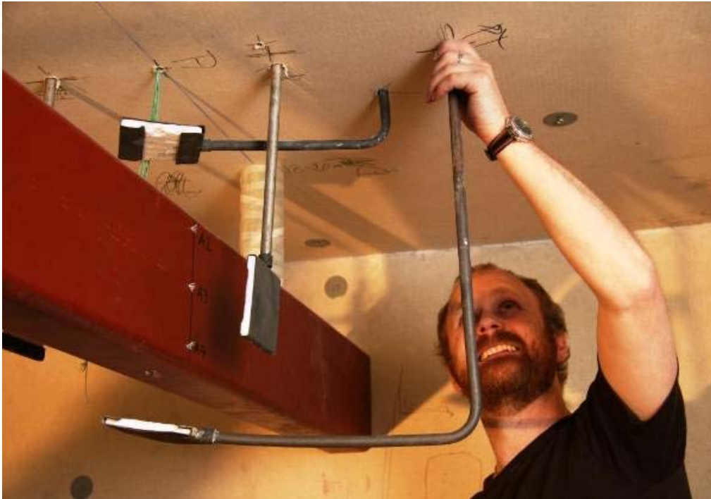
Figure 13 The plate thermometers were mounted with pipes through the ceiling. The PT thermocouple wires were drawn inside the pipes.
