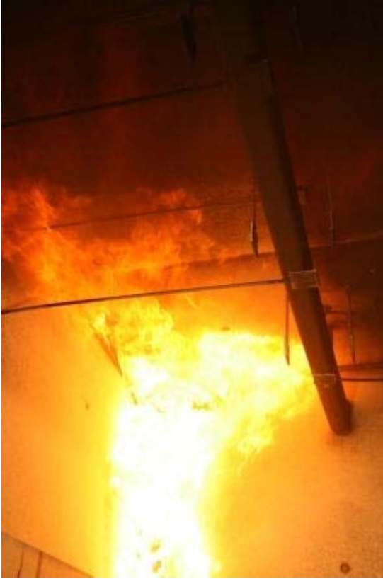
Figure 14 Fire plume and square section steel beam mounted 20 cm under the ceiling. Plate thermometer aiming at four directions are mounted at three measuring stations A, B and C.
